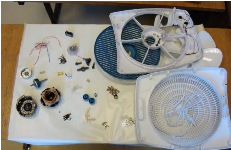
Figure 4-3: Disassembly photo of fan 5 (Box Fan)
